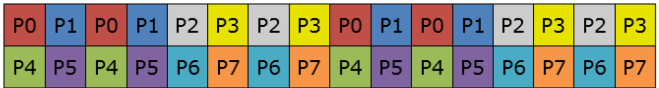
Figure 3. benchio data layout: example 3D decomposition, 2x2x2 grid per processor. Equivalent to layout of output file. Note: data is an entirely contiguous 1x32 array, split into two rows in this figure only for legibility. Contrast with the IOR parallel data layout shown in Figure 1.
